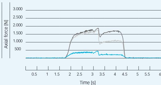
**Summary** The axial forces increase with increasing speed. With a rigid colletholder, the forces occurring when forming threads are considerably higher than with the Softsynchro® tapping holder. This allows for the optimum use of the synchronous spindle with the best possible service life and thread surface quality.
