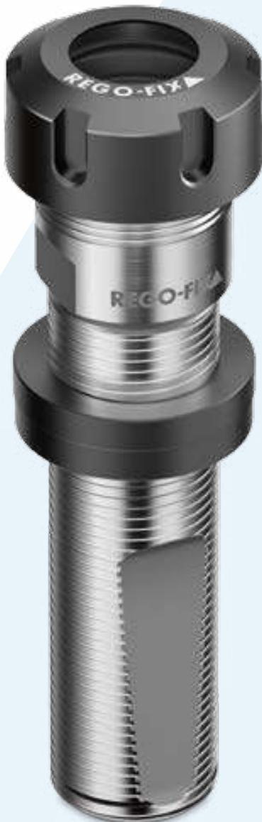
**Applications** Automotive shank colletholders with trapezoidal thread are supplied with a setting nut. With this type of colletholder, ER, ER-GB and PCM ET1 collets can be used.
