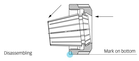
**General advice** Never clamp oversized tool shanks. For example, never use a Ø 12 mm to 11 mm collet to clamp a Ø 12.2 mm shank. Rather use the next bigger collet (in this case a Ø 12.5 mm – 11.5 mm or 13 mm – 12 mm collet). Insert tool to the full length of the collet for best results if possible.
