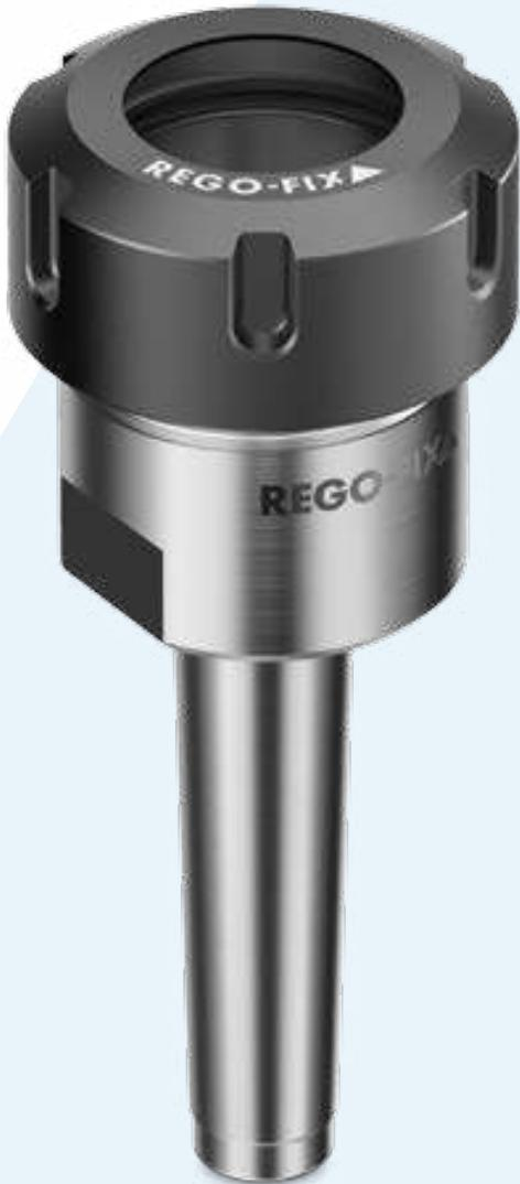
**Applications** Morse taper colletholders are designed for drawbar thread application. They can be used on milling or combined drilling-milling machines as well as on boring machines. For drilling machines we supply the corresponding tangs (ATL) on request.
