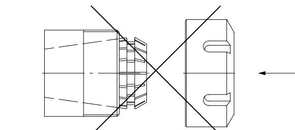
Also, never insert the tool less than  $\frac{2}{3}$  of the collet length. Improper tool insertion can permanently deform the collet and will result in poor runout.
