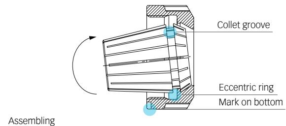
**Disassembly instructions** After the nut is unscrewed from the colletholder, press on the face of the collet while simultaneously pushing sideways on the back of the collet opposite the mark, until it disengages from the clamping nut.
