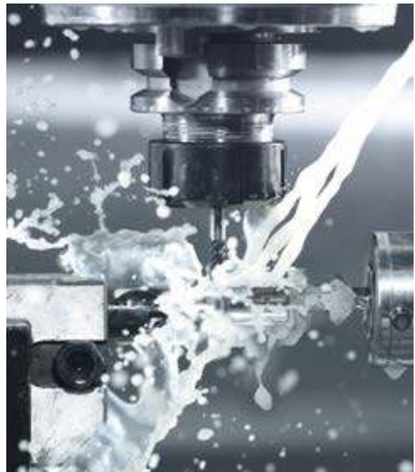
The cutting edge is subject to thermal strains. Wet machining thus helps to regulate the impact of high heat that occurs during milling, ultimately protecting the tool against total tool failure.
